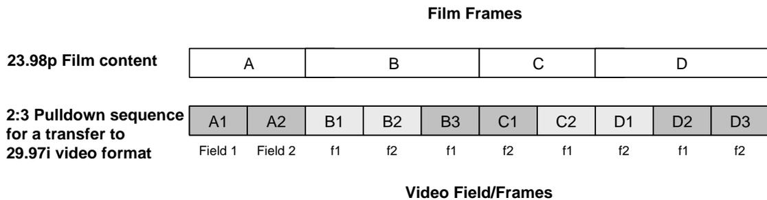
This 2:3 sequence shall be respected not only for transfers on telecines but also for frame rate conversions performed with any other system (standard converters, non-linear editing systems, etc.). It will ensure a fluid perception of movements.
