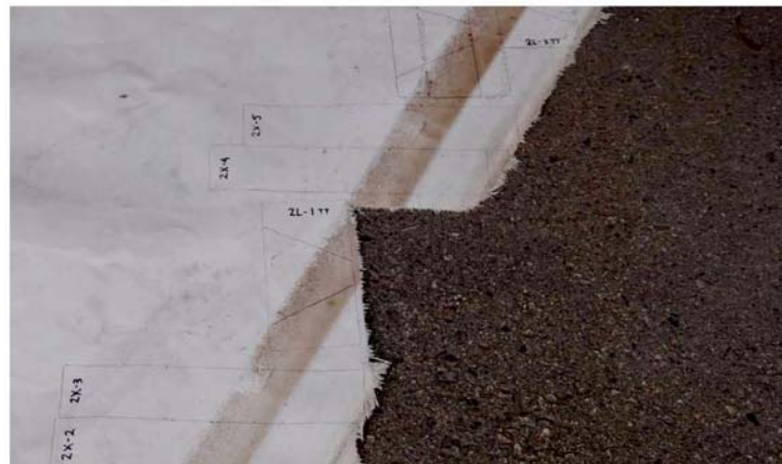
Figure E4-2: Samples 2X, 2L-TT Triangular notch does not correlate with anything on adjacent fabric segment. This was possibly removed by a souvenir hunter prior to recovery by BC Place staff.
